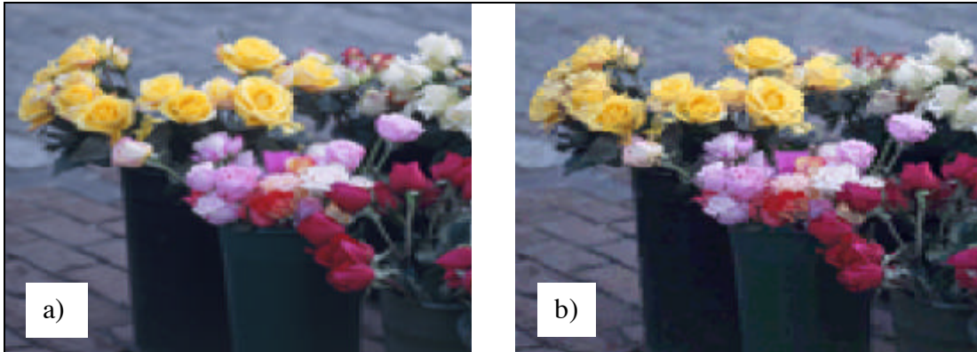
Figure 1: On the left, an uncompressed 128x128 texture; on the right, its compressed S3TC RGB DXT1 counterpart (Minification and magnification filter set to GL_NEAREST)
