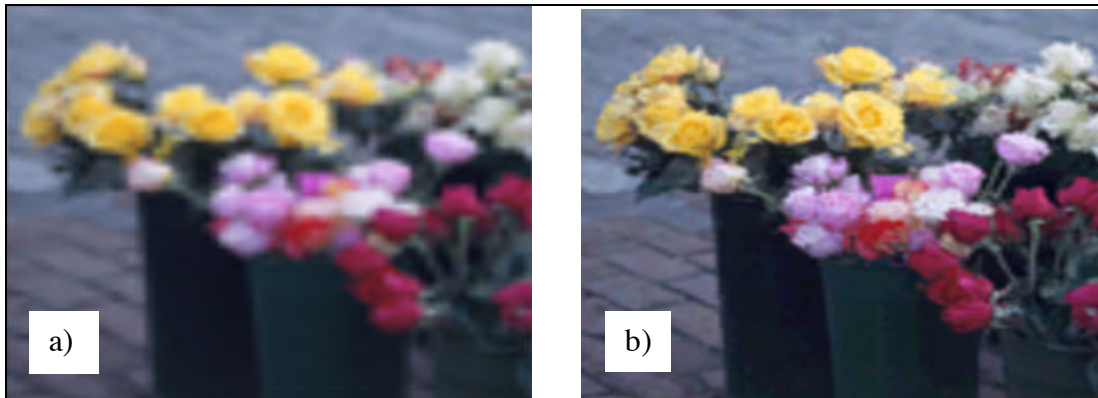
Figure 5: On the left, an uncompressed 64x64 texture; on the right a compressed RGB_DXT1 128x128 sibling (Minification and magnification filter set to GL_LINEAR). One should notice that those two textures take the same amount of memory, but the compressed version appears much sharper.
